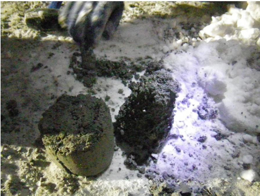
Photo 8: First attempt at core sampling. The core crumbled as it was removed from the drill bit.
